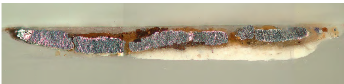
Fig. 7 – Cross section of well-preserved yellow glazed tin foil from the border edging of the loincloth of the Urnes Christ figure. 100x. (Photo: Kaja Kollandsrud © MCH, UiO)
